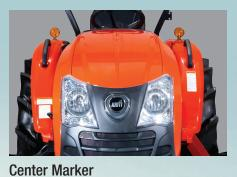
The center ridge marker on the hood assists with maintaining straight lines during operation.
