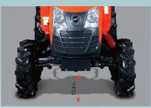
High Ground Clearance The minimum ground clearance of 13.4 in. provides sufficient clearance for use on rocky or uneven terrain.
